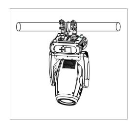
Step one: Installation the clamp onto the omega bracket;
